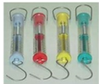
Newton Metre 1kg pulls with a force of 10N
